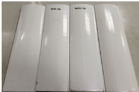
Picture: Coated wooden spruce boards after one year of outdoor weathering
