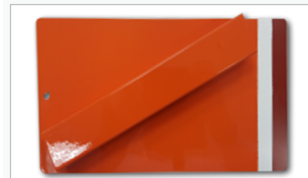
Figure 3: Orange high-gloss topcoat RR 3.3894-06 on steel
